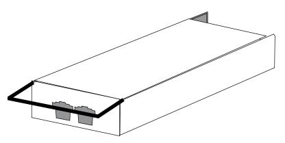
Figure 21: CFP2 LR4 Optical Module (Bail Latch Open Position)
